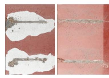
Scribe Test comparison: Commercially available liquid-epoxy based coating vs AMP-UP TM 100 (2000 hrs in salt spray chamber ASTM B117)
